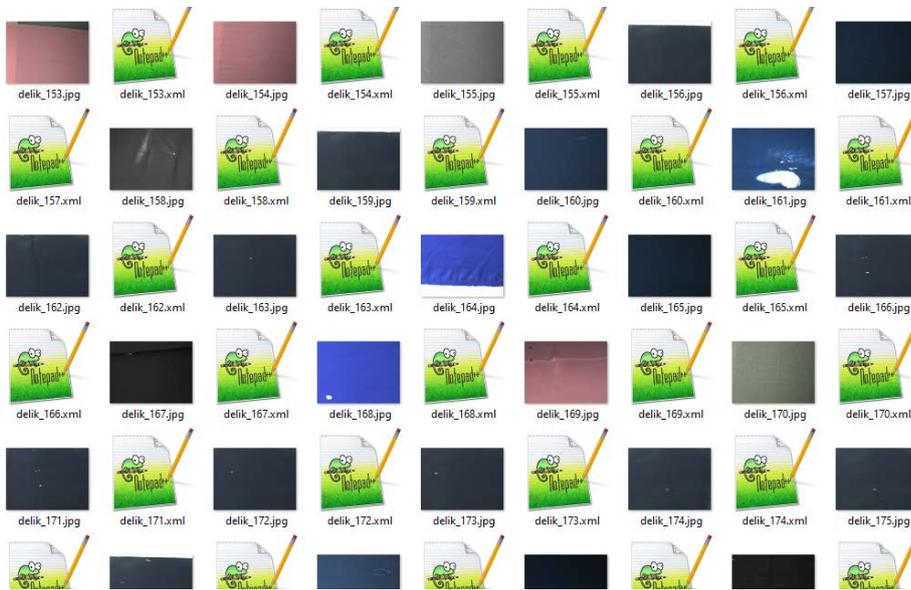
*Figure 14: Generating XML files Containing Tag and Fault Coordinates*
