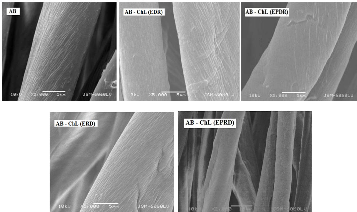
Figure 3: SEM images of alkaline scoured and bleached surface (AB) and treated with chitosan (AB-ChL) using different applying techniques EDR, ERD, EPDR and EPRD
