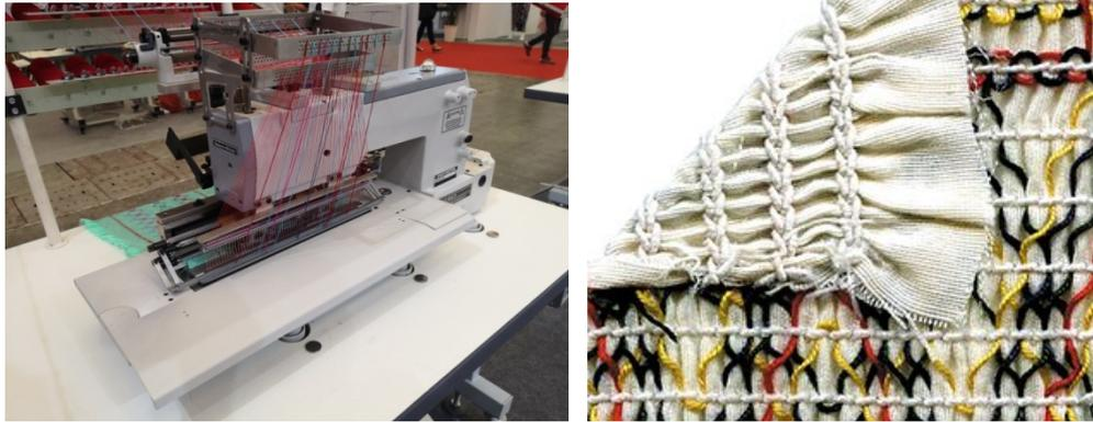
Figure 11. Multi needle shirring and smocking machine (a) and shirred and smocked fabric sample (b)
