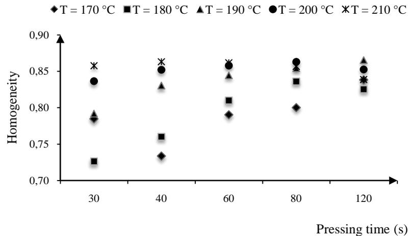
Figure 3: Homogeneity GLCM parameter of sublimation prints obtained at different temperatures and pressing times
