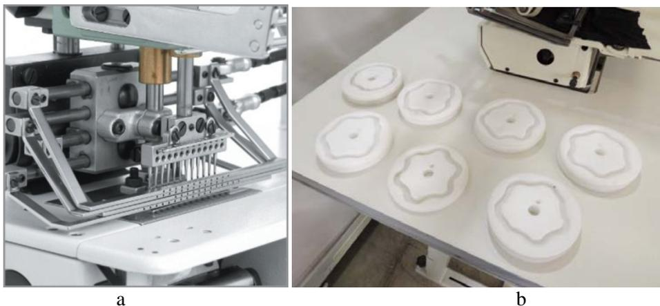
Figure 12. Thread push roads (a) and pattern cams (b)
