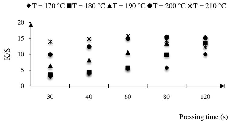
Figure 1: Color strength of sublimation prints obtained at different temperatures and pressing times
