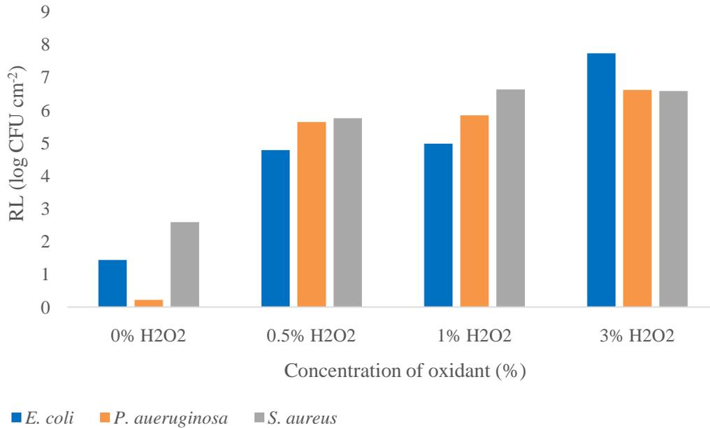
Figure 1: Disinfection activity, RL (log CFU cm<sup>-2</sup>), of 0%, 0.5%, 1% and 3% HP added in the main wash cycle against tested bacteria *E. coli*, *S. aureus* in *P. aeruginosa*
