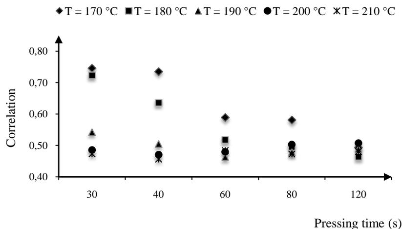
*Figure 6: Correlation GLCM parameter of sublimation prints obtained at different temperatures and pressing times*
