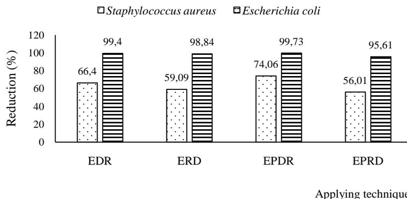
Figure 4: Reduction percentage against *Staphylococcus aureus* and *Escherichia coli* of alkaline scoured and bleached cotton yarns treated with chitosan using different applying techniques
