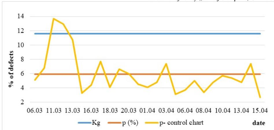
Figure 4: p- control chart, machine 2, all shifts
