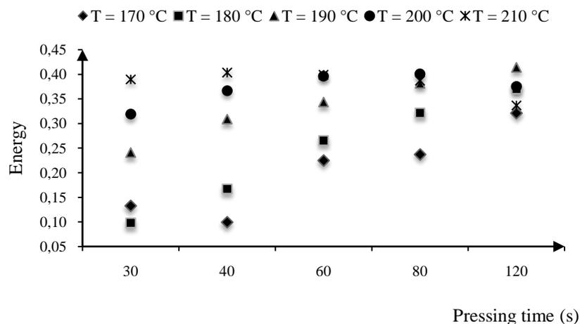
Figure 4: Energy GLCM parameter of sublimation prints obtained at different temperatures and pressing times
