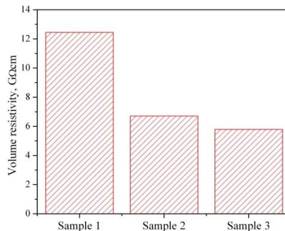
Figure 1: Volume resistivity of the knitted fabrics
