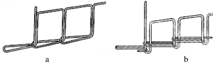
Figure 2. Stitch type 101 (a) and stitch type 401 (b)
