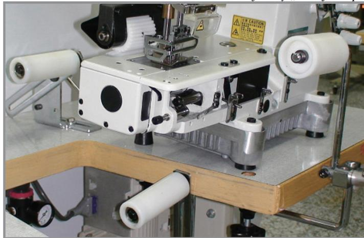
*Figure 7. Tension rollers on a machine*
