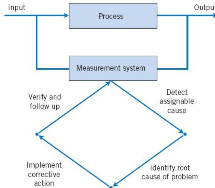
Figure 1: Process improving by application of control cards
