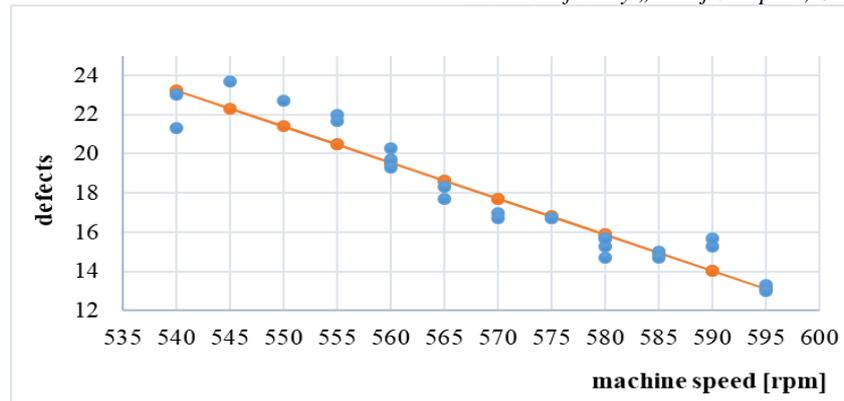
Figure 1: Regression between knitting speed and occurred defects
