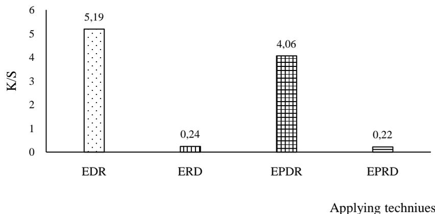
*Figure 2: Amount of amino groups onto alkaline scoured and bleached cotton yarns after treatment with chitosan using different applying techniques*
