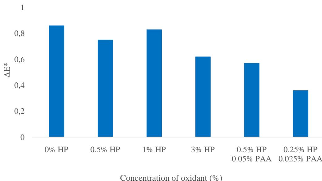
Figure 3: Colour difference,  $\Delta E^*$ , between blue cotton fabric washed with liquid detergent only and those washed with liquid detergent and added hydrogen peroxide and peroxyacetic acid of different concentration
