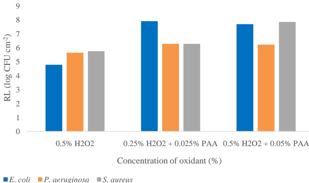
Figure 2: Disinfection activity, RL (log CFU cm<sup>-2</sup>), of 0.5% HP and a combination of HP and PAA in 0.25%+0.025 or 0.5+0.05% added in the main wash cycle against tested bacteria *E. coli*, *S. aureus* in *P. aeruginosa*
