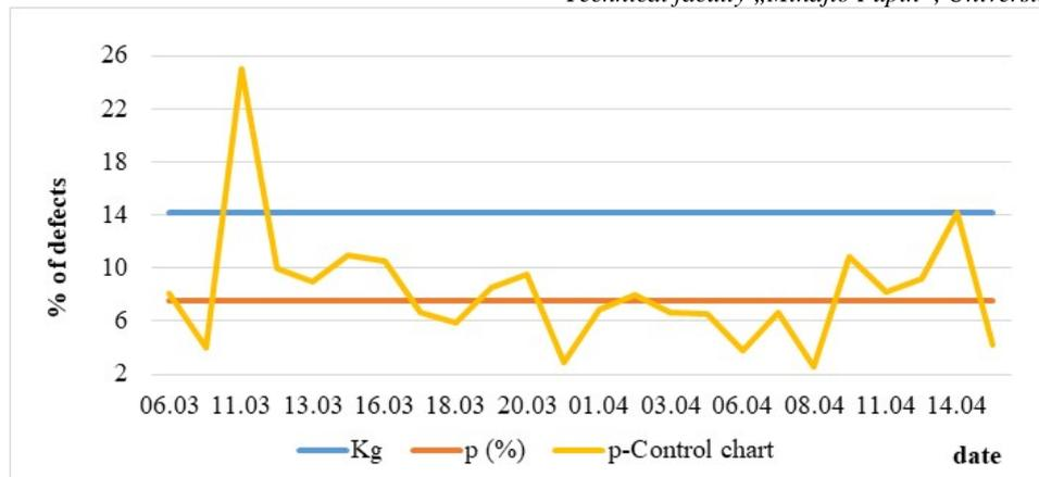
Figure 2: p- control chart, machine 1, all shifts
