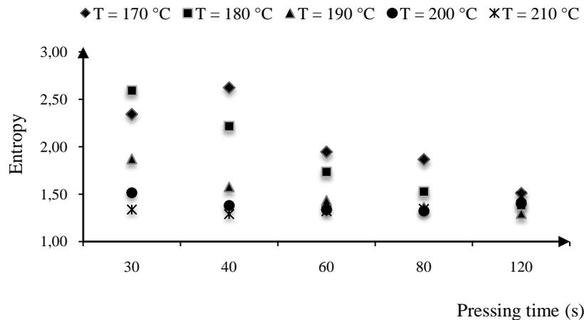
*Figure 5: Entropy GLCM parameter of sublimation prints obtained at different temperatures and pressing times*
