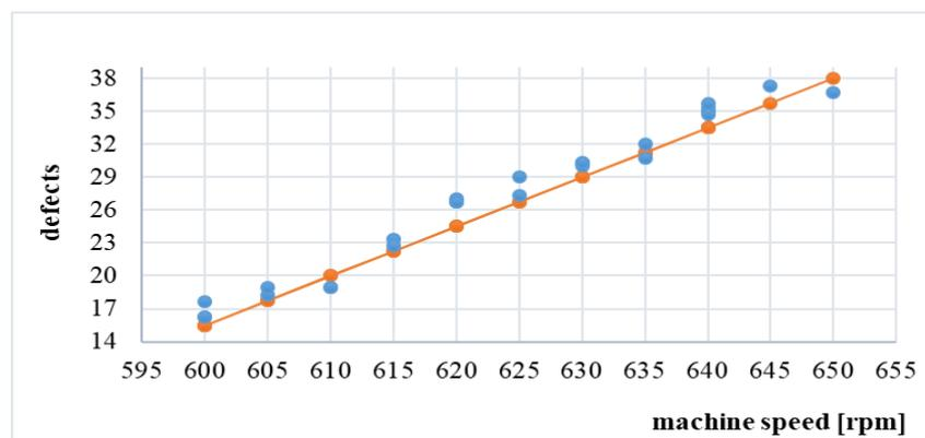
Figure 2: Regression between knitting speed and occurred defects
