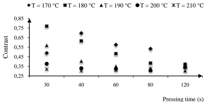
Figure 2: Contrast GLCM parameter of sublimation prints obtained at different temperatures and pressing times
