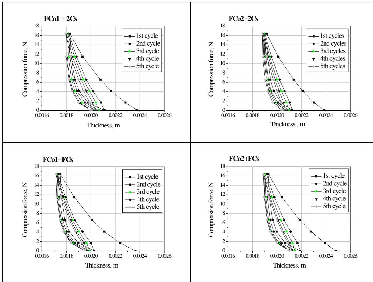
Figure 1: Compression-release curves for five successive cycles
